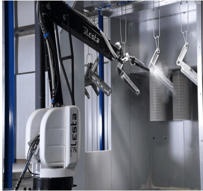
some challenges. We have made changes to how we rack parts in order coat them effectively, material usage went up through our trial and error period, and not every part is the right candidate for robot coating. We are pushing these robots harder than they ever have been pushed as we currently operate them for about 116 hours per week.
